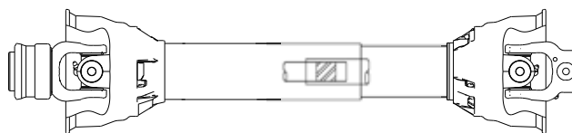
End Yokes Properly Aligned
